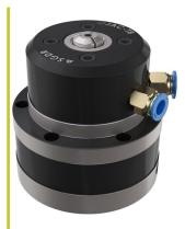
JAC-T8 is a small air collet chuck with rotary, no needto add a pneumatic or hydraulic cylinder, small OD 85mm., different workpieces to replace the collet, Clamping range 0.35-8mm, maximum speed 3500 RPM, Accuracy lessthan 0.01mm, clamping repeatability less than 0.015mm, Dustproof and waterproof design, widely used in a variety of small parts processing, such as medical Equipment, precision parts processing, grinding machine and so on.
